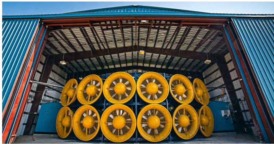
Figure 1. 12-fan Wall of Wind System, Florida International University
